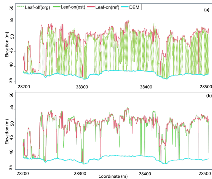
Figure 7: Sample of DSM and DEM data profiles with the depth of 0.2 m are compared, (a) before estimation and (b) after estimation.
